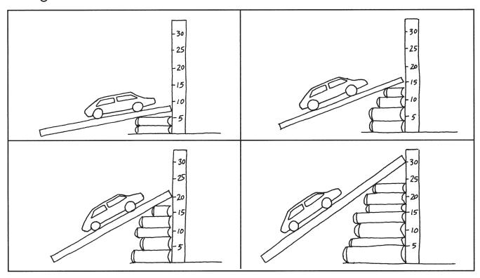
▲ Measure the distance from the end of the ramp to where the car stopped and record your results on the chart below.
