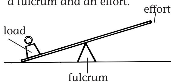
The **fulcrum** is the fixed point around which the lever turns. The **effort** is the force doing the moving. The **load** is the force that has to be moved.
