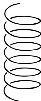
A spring can be either stretched or compressed, but it will tend to go back to its original shape. So it pulls when stretched and pushes when compressed.
