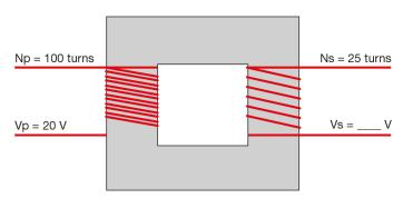
ii Calculate the current in the secondary coil, knowing that  $I_p = 3A$ .
